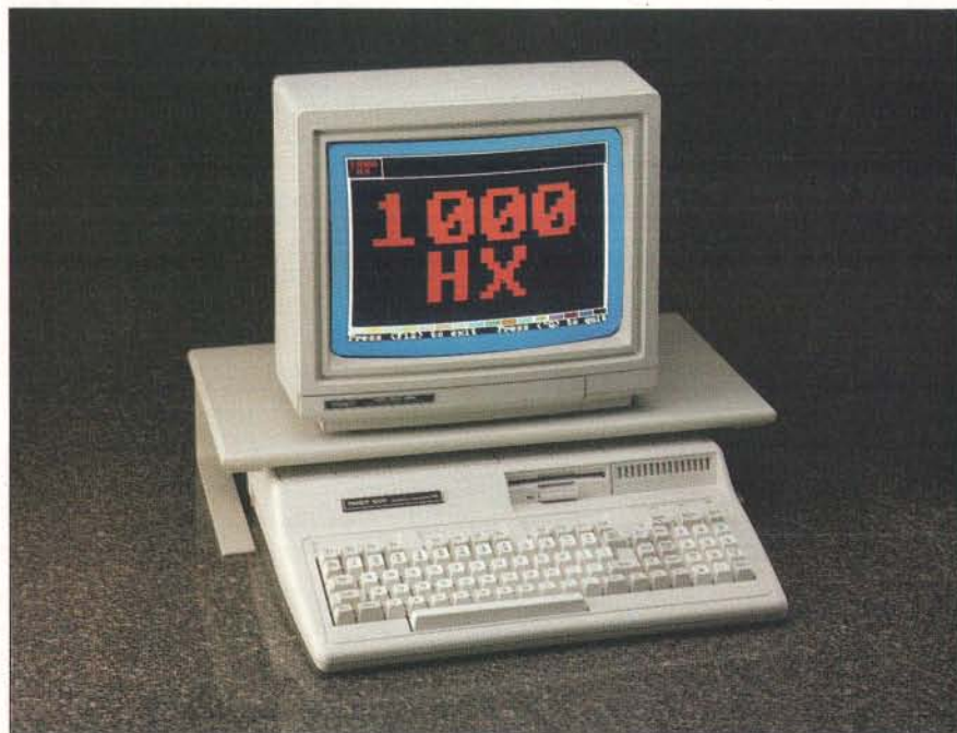
Photo 4: The Tandy 1000 HX, an 8088-based machine with MS-DOS in ROM.
